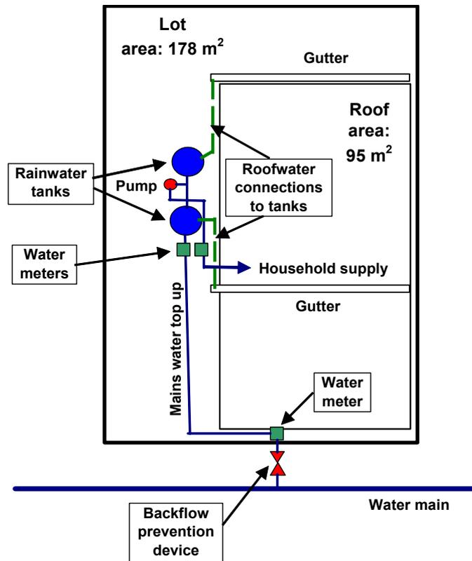
Figure 1: Plan view of the dual water supply solution at Carrington
