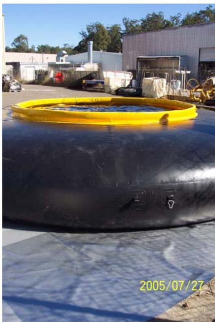
**Reo Sac®** Onion tanks are self-erecting. A "floating collar" enables them to rise to the maximum fill height as they fill. The key advantage of a **Reo Sac®** Onion tank over a pillow tank is the ability to fill and empty it faster than a standard pillow bladder tank. This is due to the large opening aperture within the floating collar.
