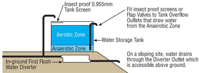
After rainfall when an In-Ground Diverter is installed, not only will the diverter chamber empty, the water held in underground pipes will also drain out through the diverter, converting it to a “dry” system.
