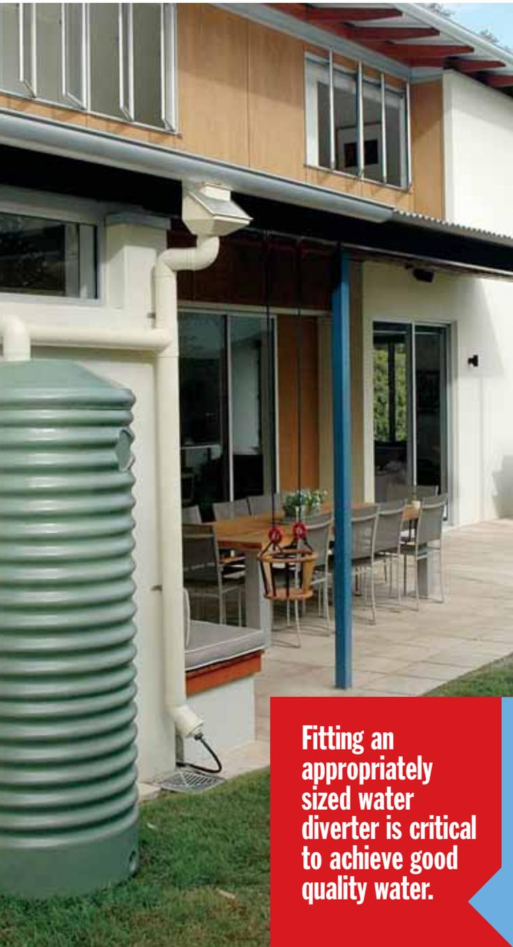
**Fitting an appropriately sized water diverter is critical to achieve good quality water.**
